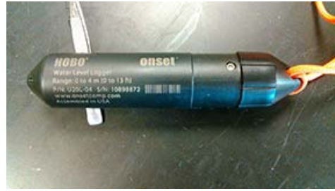
Fig. 4b. An ONSET HOBO U20L-004 data logger. Each pair of data loggers measured hourly water and air pressure to calculate hourly stream stage (height), and air and water temperatures.
